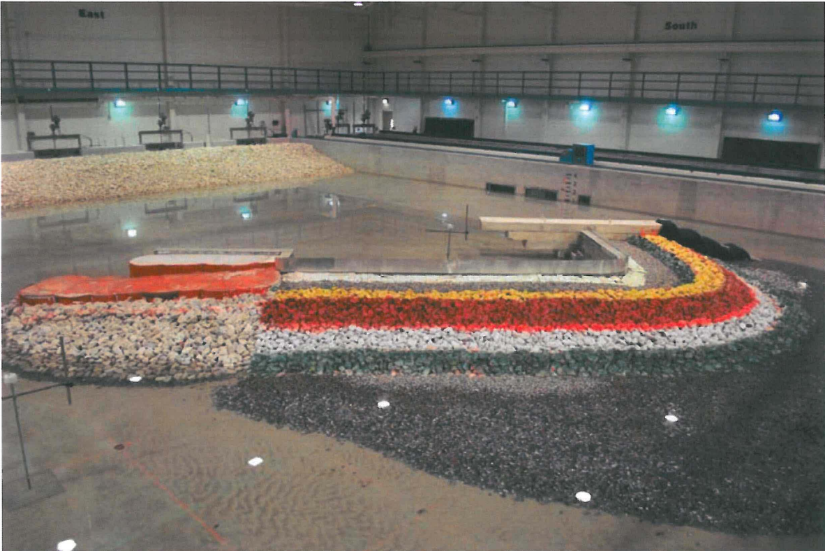
Figure 7. Shore Protection Model in 3-D Wave Basin at 1:20 Scale – Texas A&M University
