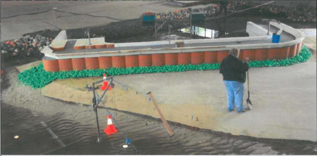
Figure 8. OPEN CELL® Bulkhead model in 3-D Wave Basin at 1:20 Scale – Oregon State University
