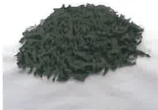
FIGURE 5 BioConERS Dried Biosolids (prior to incineration)
