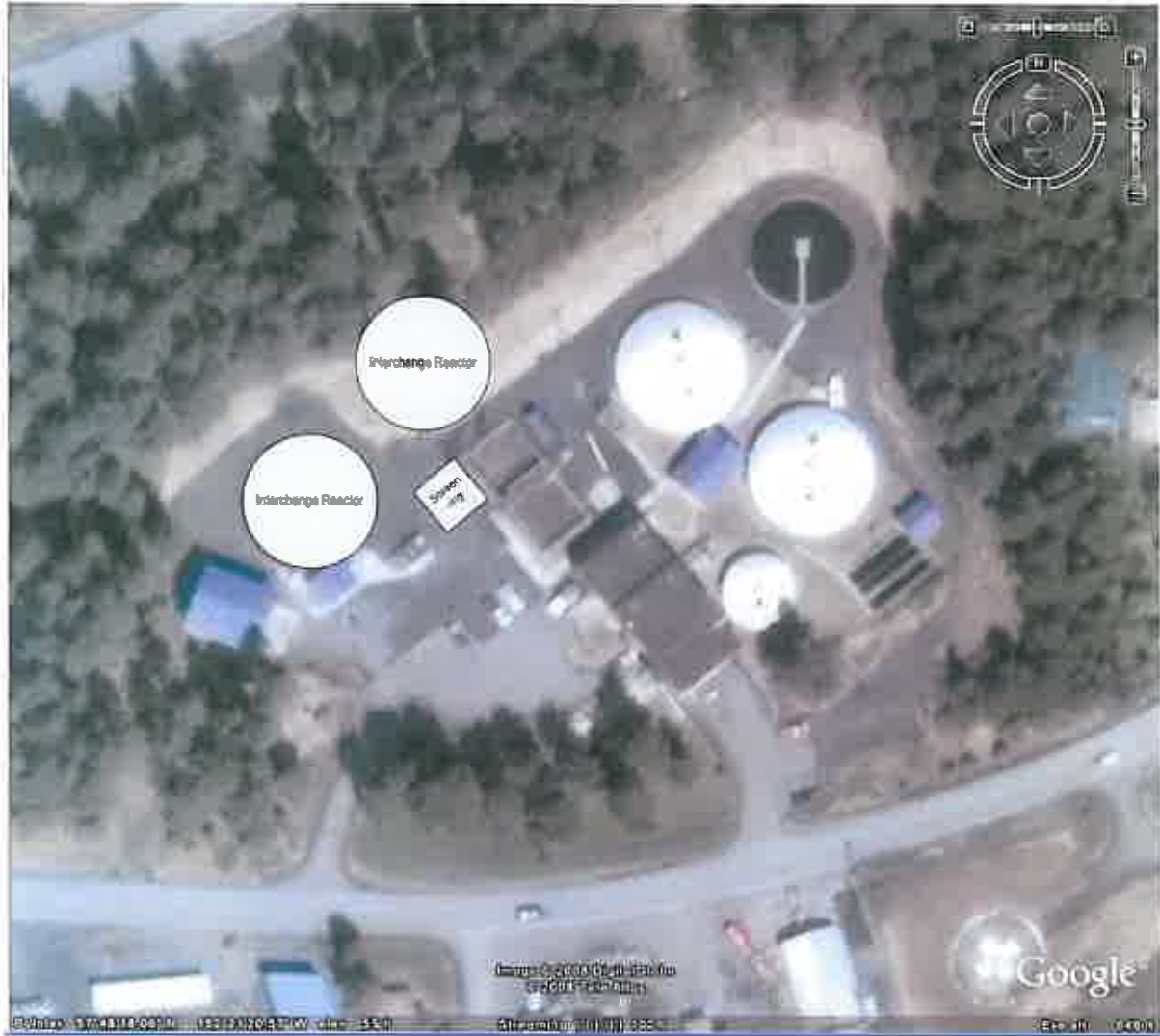
FIGURE 2 Preliminary Site Layout for Cannibal Process
