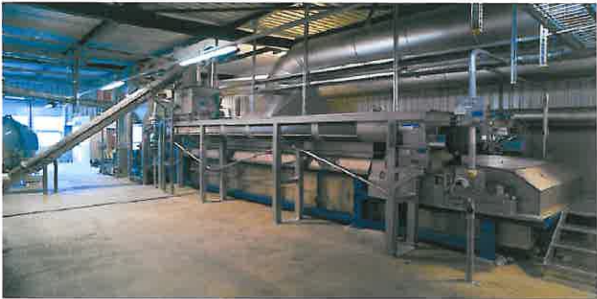
FIGURE 9 Belt dryer layout in Wohlen, Switzerland.
