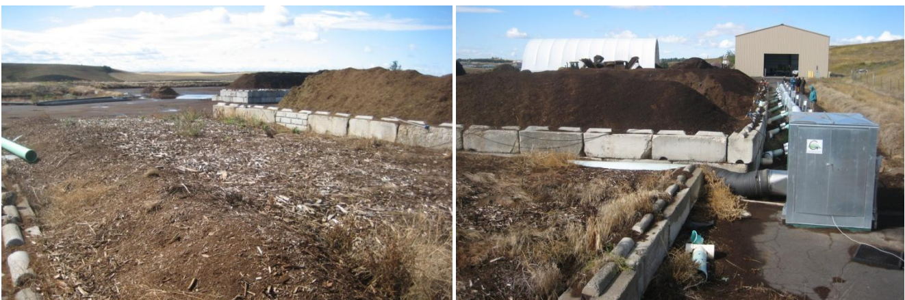
Figure 4 - Aerated Static Pile System at Washington State University with Biofilter in Foreground
