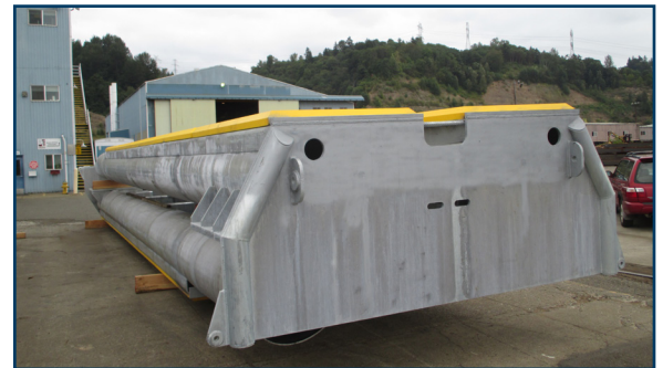
Galvanized fenders with UHMW panels waiting for metalizing on cap plate tops.
