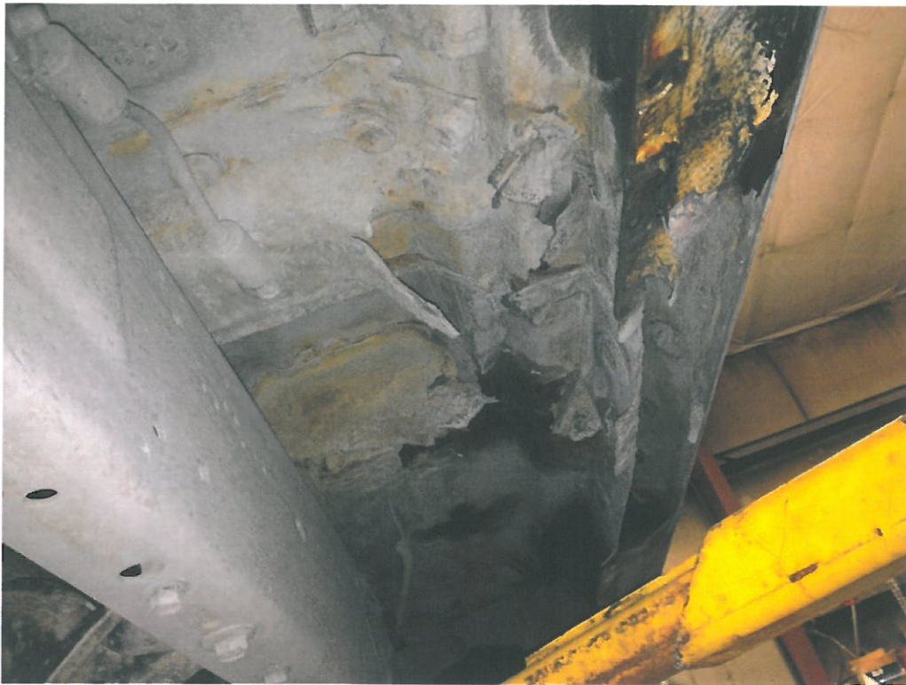
Cab rusted through, passenger side
