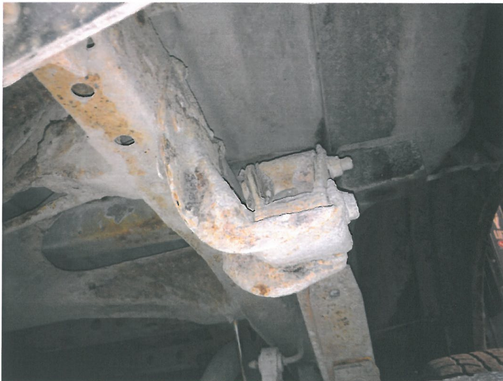
Spring shackle mounts heavily rusted
