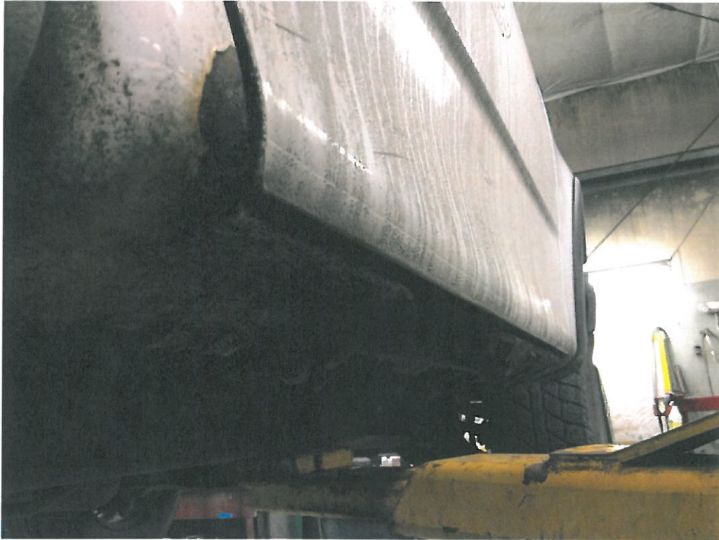
Cab rusted through, passenger side
