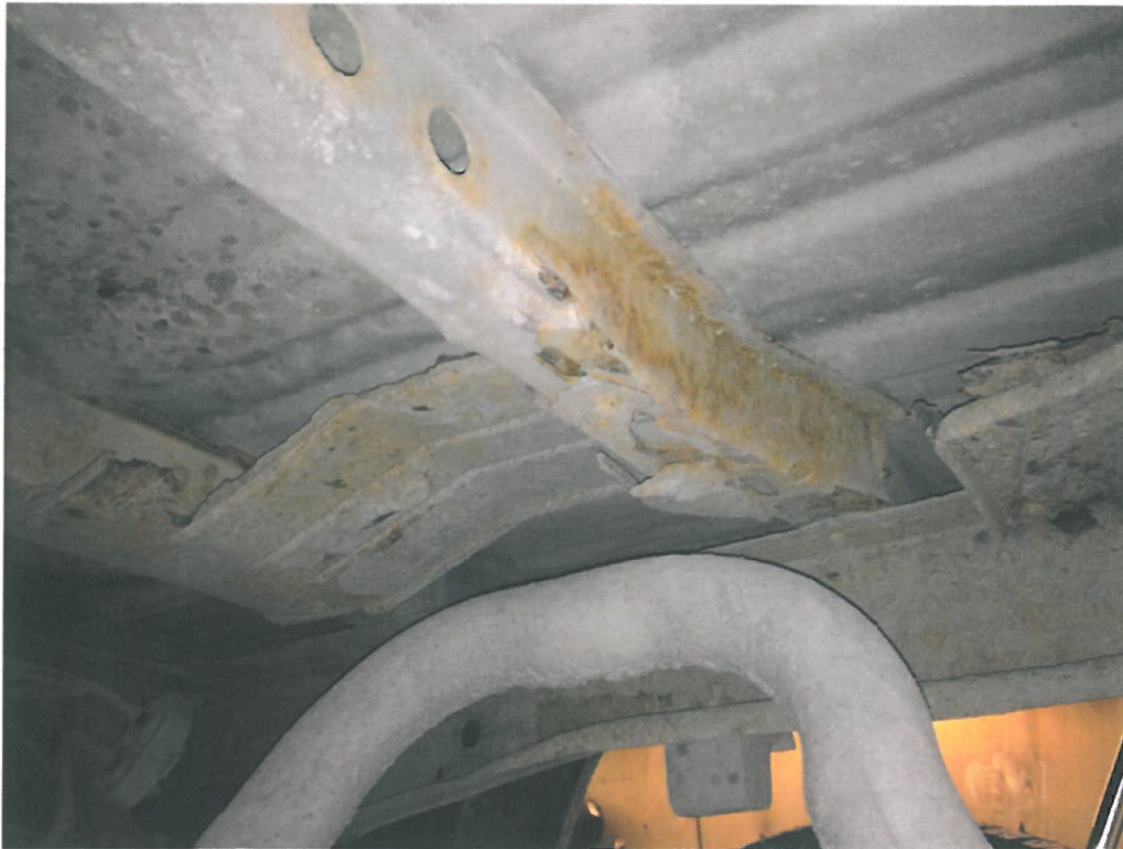
Bed supports rusted through
