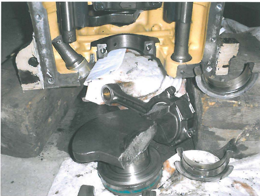
Auxiliary engine with broken crankshaft and block
