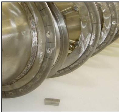
Scroll with tungsten carbide wear tiles
