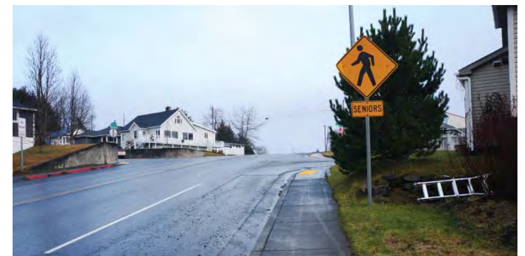
Image 27: As noted in the “Other Comments” row there is a pedestrian sign for crossing Rezanof Drive at the intersection of Mill Bay Road. But as seen in this image the crest in the hill above this crossing makes it hard see oncoming traffic.
