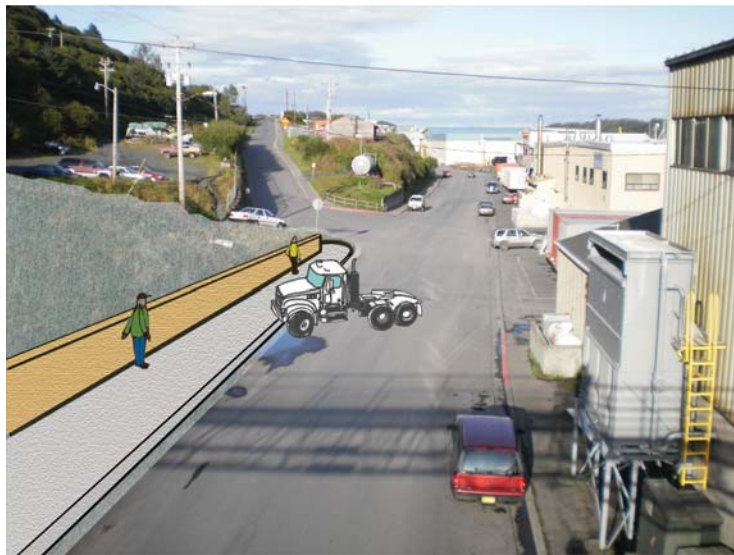
Shelikof Street: 8' sidewalk and retaining wall.
